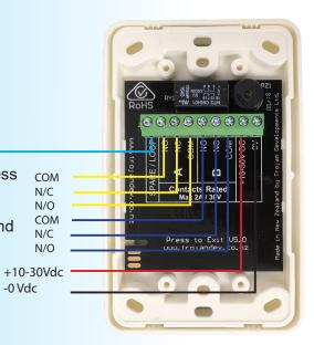
Spare / Loop terminal for other terminations Set "A" Contacts connect to the Request to Exit input on the Access Control door module. You might need an EOL resistor.
